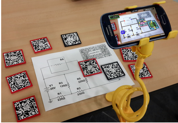
Fig. 1. Virtual Circuits basic setup: The AR GUI and simulation engine run on the mobile device while a sheet of paper and a set of plastic tokens serve as the simulation's TUI.
