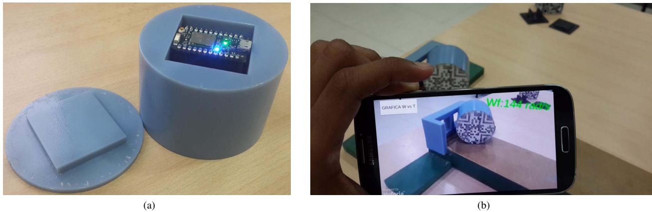
Fig. 9. Our next Smart Object prototype, the Smart Cylinder, allows students to explore the concepts of angular momentum and acceleration in a rotating body.
