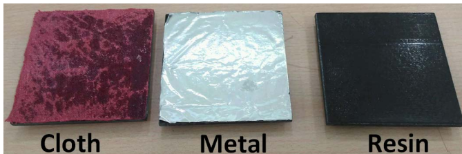
Fig. 6. The Smart Cube has a detachable bottom cover that acts as the contact surface while sliding. During laboratory activities, students measured the friction coefficient of three different contact surfaces : metal, cloth, and resin.
