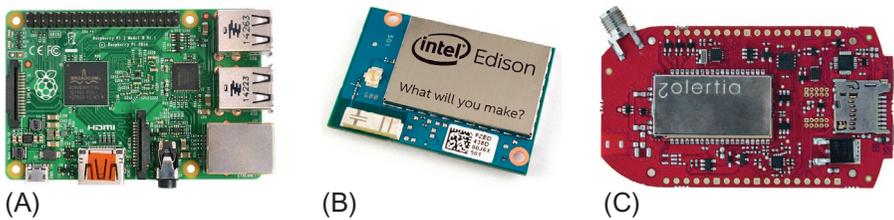
**Fig. 8.6** Sensor nodes can be divided into three categories: single-board computers (SBC) (A), high-end ESM (embedded sensor module) (B), and low-end ESM (C).
