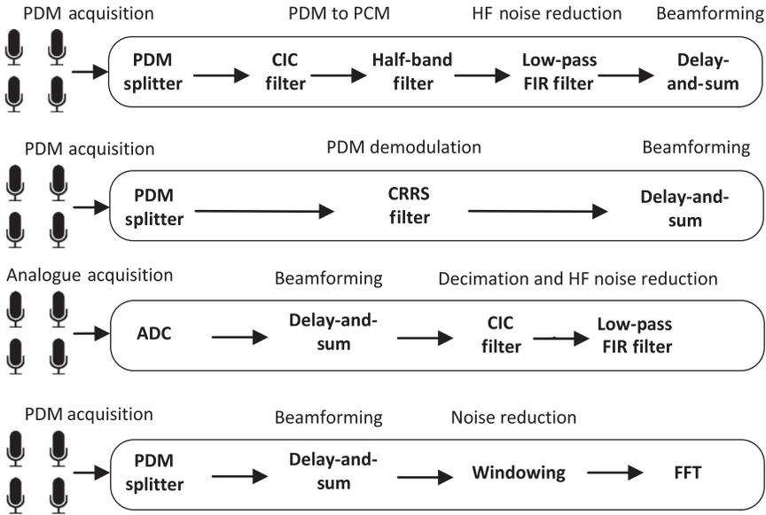
Fig. 8.7 Signal processing strategies for MEMS microphone arrays implemented on FPGAs.
