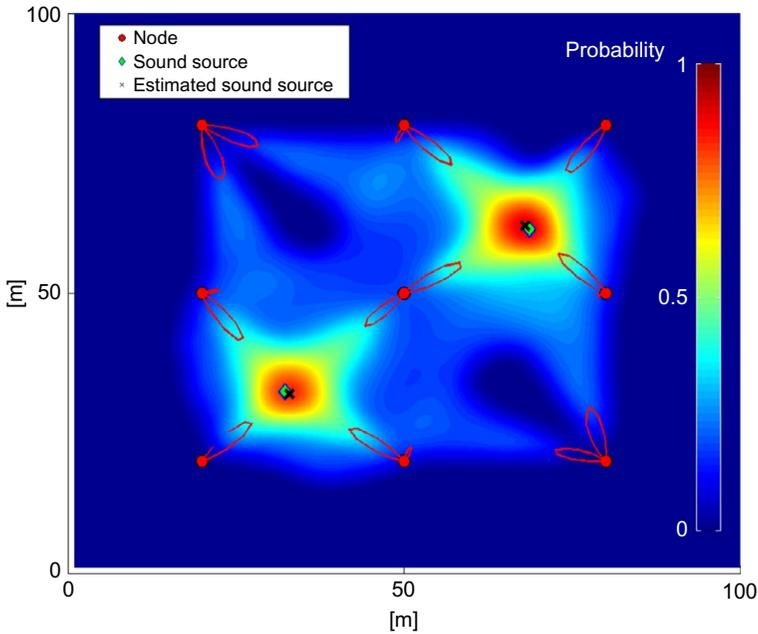
**Fig. 8.8** Each WSN node uses an on-board microphone array to estimate the direction of nearby sound sources (*red lines*). These estimations are then combined to form a probability map of the possible geographic location of all sound sources.
