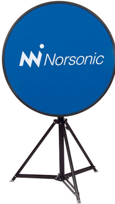
**Fig. 8.3** The Norsonic Nor848A 0.4 m diameter acoustic camera, which uses a 128 MEMS microphone array to graphically represent the surrounding soundscape.
