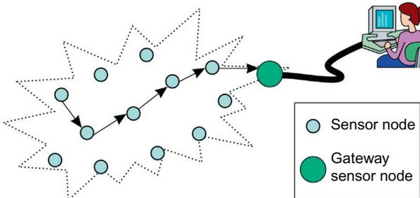
**Fig. 8.5** Sensor nodes in a wireless sensor network (WSN) measure environmental parameters and transmit the data back to a network gateway where it is aggregated, stored, and processed.
