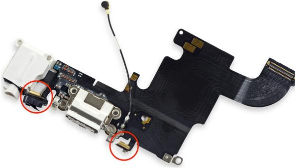
**Fig. 8.2** iPhone 6s lightning cable assembly, with two MEMS microphones circled in red.
