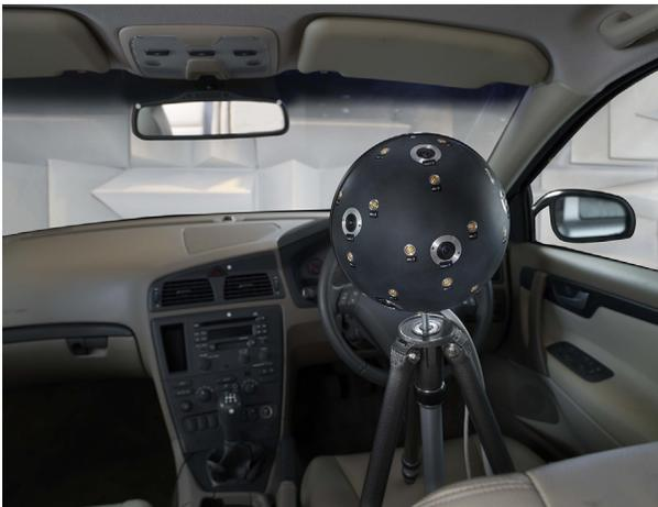
**Fig. 8.4** A spherical microphone array by Bruël and Kjør, measuring the soundscape inside a car.
