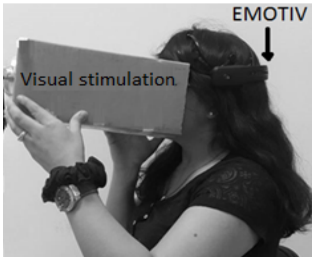
Fig. 1. Visual stimuli generated by a display with LEDs used to acquire the occipital EEG signals.
