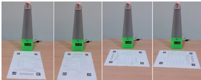
Fig. 4. A user of SARA can place the paper-based assessment in any orientation below the camera; SARA automatically corrects it.
